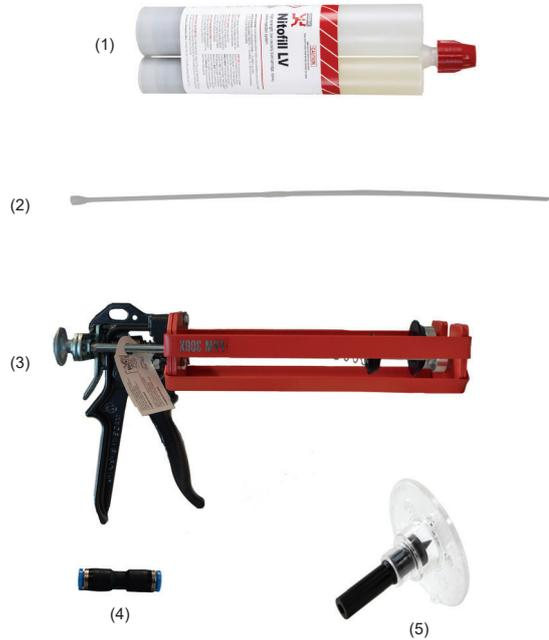
To ensure the product is mixed properly through the static mixer, always gun out a small amount of mixed Nitofill LV resin prior to attaching the outlet end to the flange.
