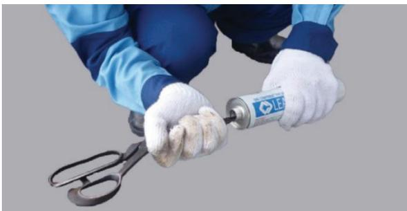
1. Break the moisture-proofing aluminium foil on top of the cartridge, and remove the metal back seamer from the bottom.
