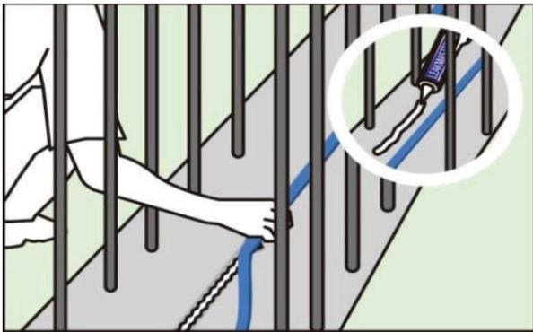
As an adhesive to the concrete before Hydrotite installation, when the surface is rough
