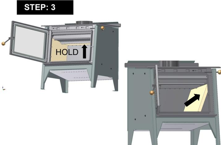
While holding up the baffle assembly horizontally, insert the opposite side brick in from underneath it, as shown above. The 2 side bricks will now support the Baffle.
