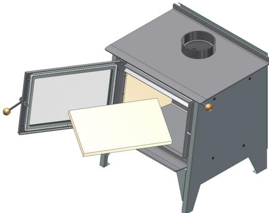
Fit back Vermiculite Board panel into the firebox back, ensuring that it is sitting hard against the back of the firebox.
